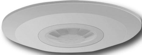
This product uses an infra-red heat detector. The detector senses 'warmth movement' in the surrounding area when it is dark. When movement is detected the sensor is activated and triggers the connected load. It has a built in photo-cell that can identify day and night.
