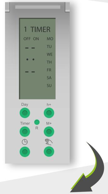
When you have finished setting the required times, press the 'CLOCK' button to confirm and revert the present time.
