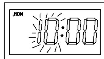
**Note: If '+' or '-' button is held for more than 2 seconds, the selected time digit will add or decrease quickly (about 5 steps per second), if no key is pressed within 60 seconds the display will return to operating mode.**
