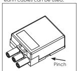
**Male Socket** Up to 2.5mm<sup>2</sup> flexible 3 core cable can be used.
