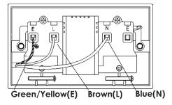
For switched sockets **M22SW** and **M22SM** follow the diagram below.
