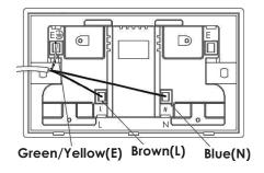
If earth conductors are bare, they must be sleeved with appropriate green/yellow sleeving.
