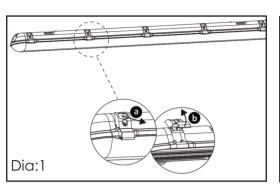
2. Press clips to remove gear tray. Take care not to touch the LED lamp. Dia:2.
