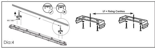
If suspended the supplied suspension clips must be used with a suitable cable suspension system, capable of bearing the weight of the luminaire. The luminaire can also be wall mounted.
