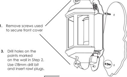
2. Hold the back cover up to the wall in the desired fixing position, mark hole positions.
