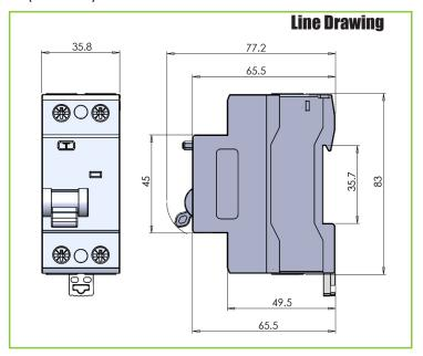
**Type A -** Tripping is ensured for residual sinusoidal alternating currents and residual pulsating direct currents, whether suddenly applied or slowly rising.
