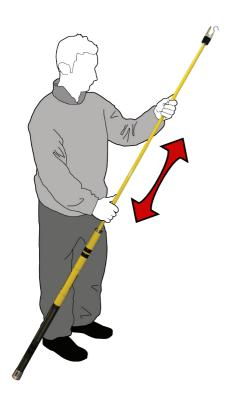
The Telescopic Pole is a series of conical tubes which interlock when extended. By sliding the section of tube out, starting with the smallest, the pole is quickly extended to the desired working length.
